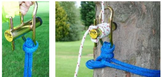
When selecting the best place to mount the device try to locate an area where there is little or no stem taper. If the tree is being removed it may be possible to achieve this by shaping the stem.
