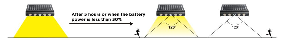
Lamp automatically lights up at night and keep 100% brightness, after 5 hours or when battery power is less than 30%, lamp turns to Energy Saving Mode: Lamp automatically turns to 100% brightness when motion is detected in the range ≤8mtrs, then turns off after 20 seconds of no motion.
