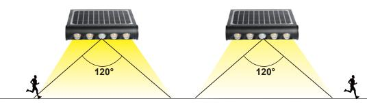
Lamp automatically lights up at night and turns to 100% brightness when motion is detected in the range ≤8mtrs, then dim to lower brightness after 20 seconds of no motion.
