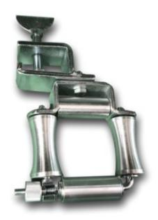
The EPD clamping roller can be clamped without tools to beams, trays or racks. Also by removing the clamp part it can be bolted directly down to Unistrut or trays etc. Fitted with a hinged gate and knurled nut, cable can easily be extracted. The cable roller is suitable for cables up to 60mm diameter with a weight capacity of 100Kg
